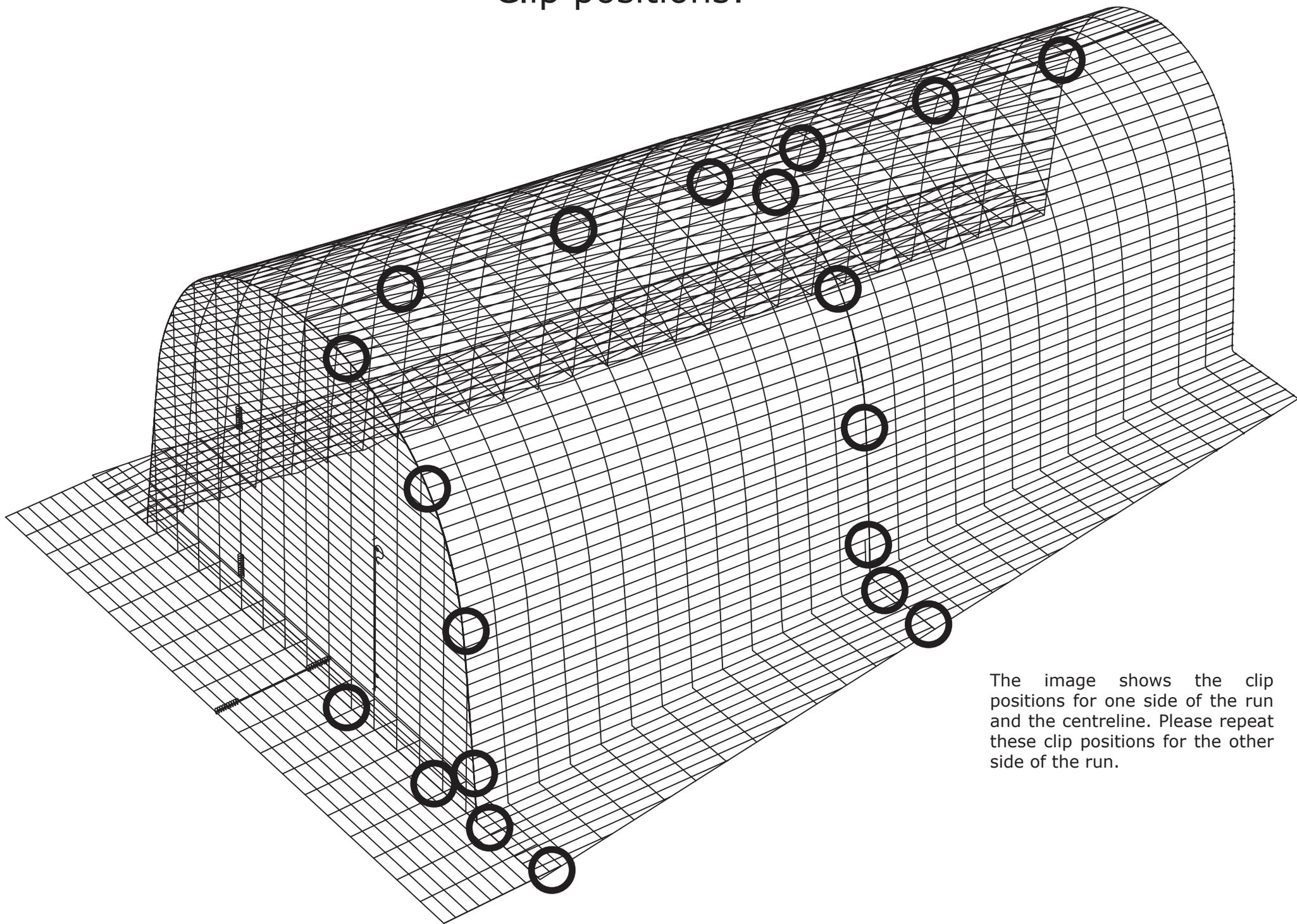
The image shows the clip positions for one side of the run and the centreline. Please repeat these clip positions for the other side of the run.
