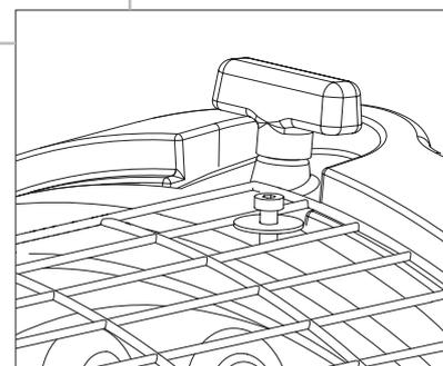
Screwing the top of the small right run panel into the base
