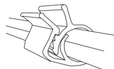
Clip securing two run panels together
