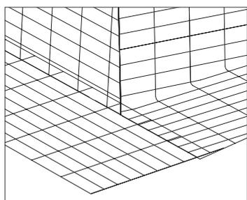
'End skirt panel' underlapping the run panels by one rectangle.
