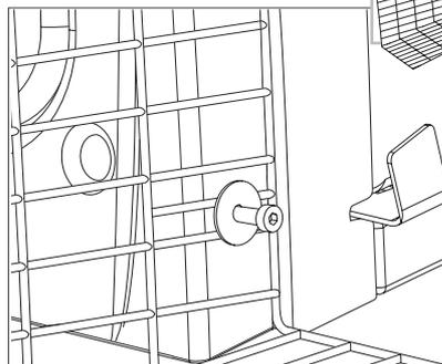
Screwing the bottom of the small right run panel into the base
