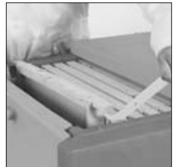
Use the curved end of the tool to lift the frame up.
