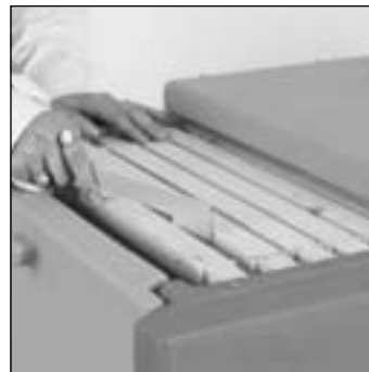
Separate the frames by levering apart with the tool.
