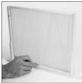
Take the piece that was snapped off earlier and mark the positions of the wires with a pen. Tap three nails in.
