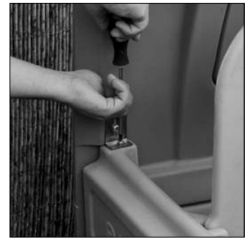
Undo the two bolts and remove the bracket.
