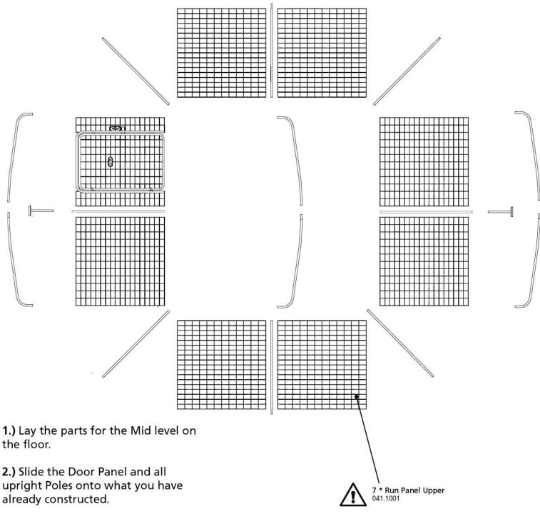
**3.)** Complete the Mid level referring to the diagram on page 8 for clip types and positions.
