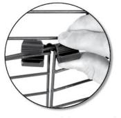
Position around the wires to be joined and squeeze both clips.
