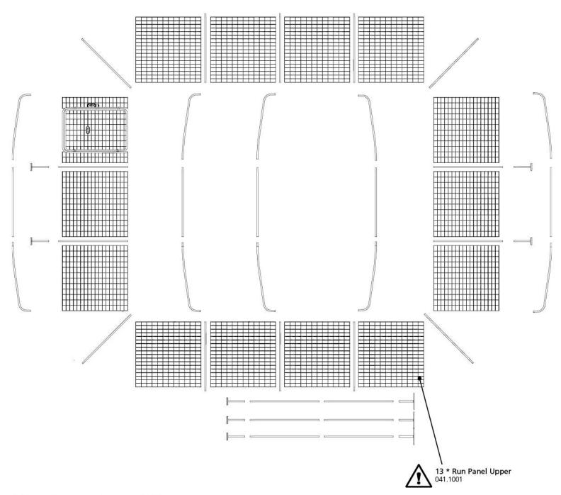
**1.)** Lay the parts for the Mid level on the floor.
