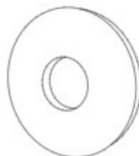
X2 Nylon Washer M6 x 18 x 1.6mm 800.0449
