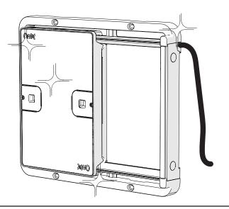
After rain in freezing temperatures, sleet or snow you may need to defrost your Autodoor to restore proper function to moving parts. To do this we recommend pouring warm (not boiling) water over any affected parts and then drying them.
